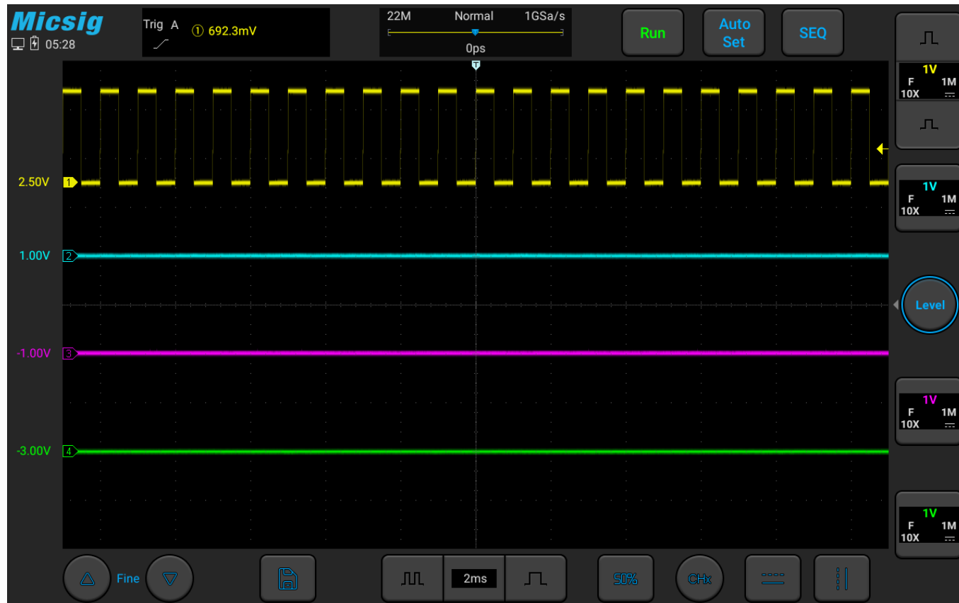
Figure 4-2 Current Channel and Non-Current Channel
