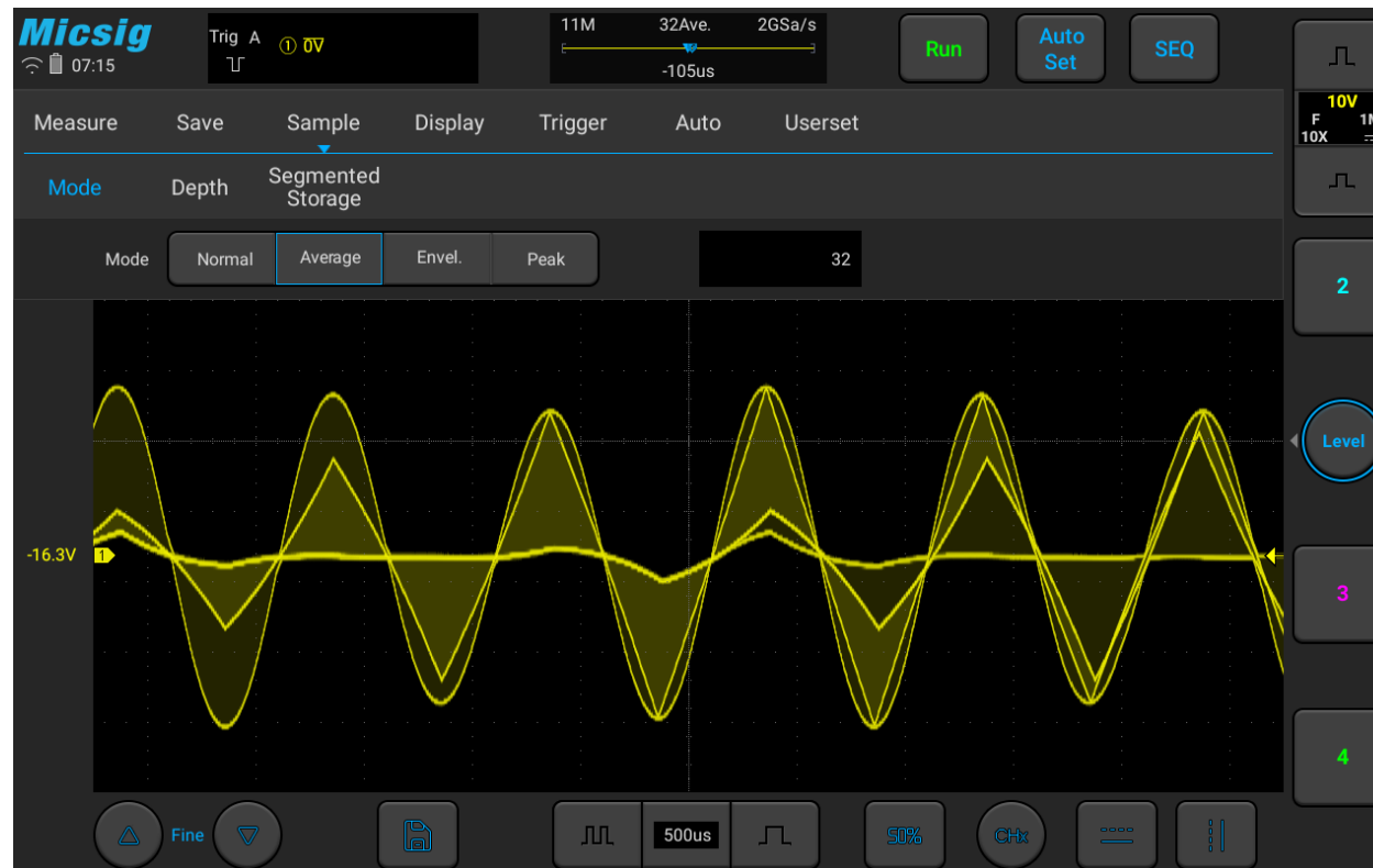
Figure 10-8 AM Signal in Envelope Sampling Mode (32)
